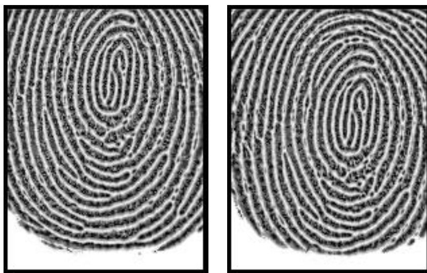
Figure 3 Fingerprint image before (left) and after (right) multiple exposure to 15kV ESD.
